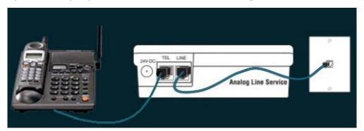
**Step 3**. Next, plug the small end of the Power Adapter into the port labeled 24VDC on the DPS3, then plug in the Power Adapter into a standard AC receptacle. Your final assembly should look like this figure below:
