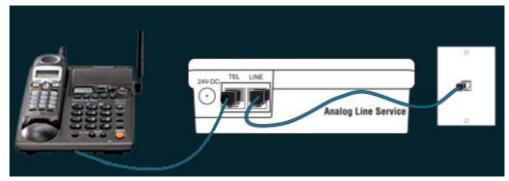
**Step 3**. Next, plug the small end of the Power Adapter into the port labeled 24VDC on the DPCB, then plug in the Power Adapter into a standard AC receptacle. Your final assembly should look like this figure below:
